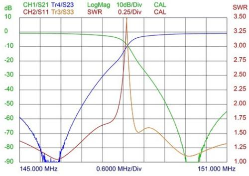
Typical response curves @ 8 MHz duplex spacing
