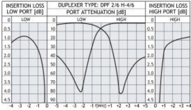
TYPICAL RESPONSE CURVES @ 9 MHZ DUPLEX SPACING
