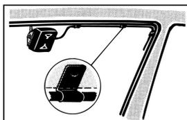
6. Fit matching unit by pressing it firmly into position. Secure cable using clips provided.
