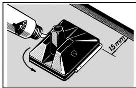
2. Fit mount to screen and press firmly. Apply glue along the edge between mount and glass.
