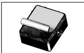
5. Remove the protective foil on the matching unit.
