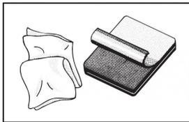
1. Clean both sides of the windscreen where the antenna mount and the matching unit are to be fitted and then remove the protective foil from the antenna mount.
