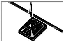
4. Fit the cover and press down firmly. After 2 - 24 hours the whip can be fitted.
