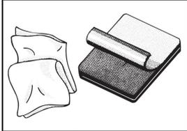
1. Clean both sides of the windscreen, where the antenna mount and the matching unit are to be fitted, and then remove the protective foil from the antenna mount.
