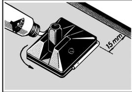
2. Fit mount to screen and press firmly. Apply glue along the edge between mount and glass.
