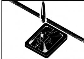
4. Fit the cover and press down firmly. The antenna whip can now be fitted.
