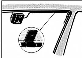
6. Fit matching unit by pressing it firmly into position. Secure cable using clips provided.
