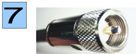
Solder inner conductor at the tip carefully.
