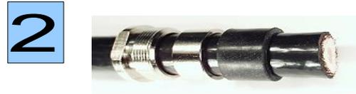
Move the nut, clamping ring and rubber washer over the cable tail. Hint: With a bit of Vaseline the rubber washer can be moved easily over the cable sheath.
