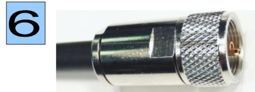
The prepared cable tail has to be carefully inserted into the housing until stop. Tighten the clamping nut finger tight with two open-ended spanners 17/18 mm. A small split should remain visible between clamping nut and connector housing.
