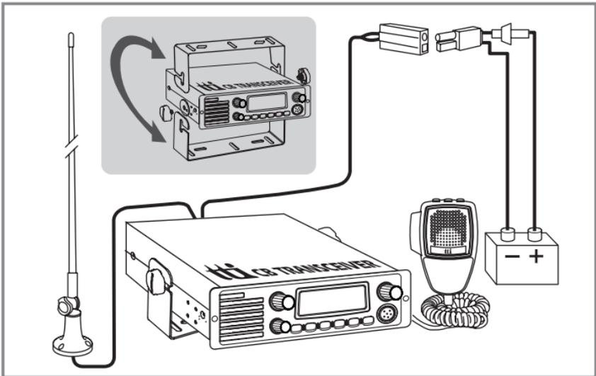
It is very important to select a good quality high efficiency 27MHz antenna. A poor quality antenna or one not designed for the 27MHz band will give very poor performance and could cause damage to the transceiver.
