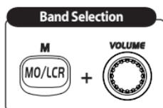
Pressing “MO/LCR” button of transceiver, turn on the transceiver. Using the channel selector, select the band that you are going to select. The LCD display offers you the band information. The band chart for each area is as follows.
